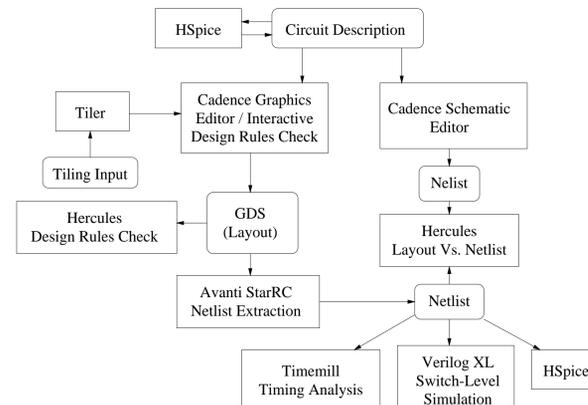
The design process comprises many steps, all of which must be completed to ensure the design will perform the necessary operations and operate as intended. This poster describes the process for only the vector datapath, which is being designed with custom logic; other parts of the microprocessor are being designed using macro blocks, synthesized logic, and other methods of design. The process is, in many steps, the same, but there are some significant differences as well.
