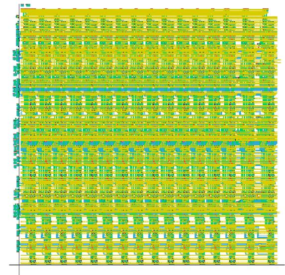
The layout of the basic block of the multiplier (which is repeated sixteen times to create the full multiplier) is complete and shown above. The circuits for all other blocks are complete, as is the layout of the gates and cells they comprise.
